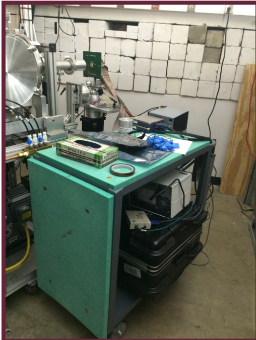
Equipment carts shielded with borated polyethylene.
